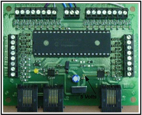
Five volts is available on the mini panel by soldering a wire to the indicated hole (above). To avoid potential damage to the mini panel or BD20 use only the 5 volts from the mini panel. There are no specific voltage or current requirements for the transistor as long as it is an NPN transistor. The 1 K resistor can be any wattage, 1/4 Watt is the most common.
